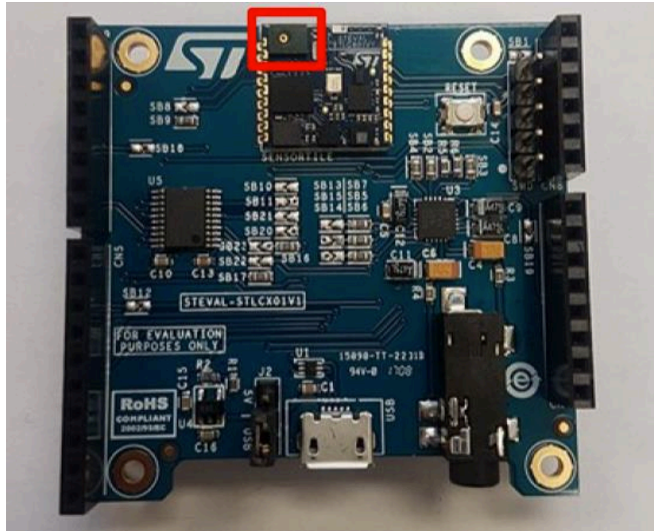
Figure 6: Ensure the orientation of the SensorTile on the larger evaluation board matches this figure. There should be a green protrusion with a little metallic hole right next to the ST logo.
