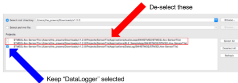
Figure 27: Only selecting one project from the existing files to import into the workspace.
